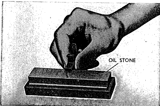
Fig. 5.24 Correction by oilstone
